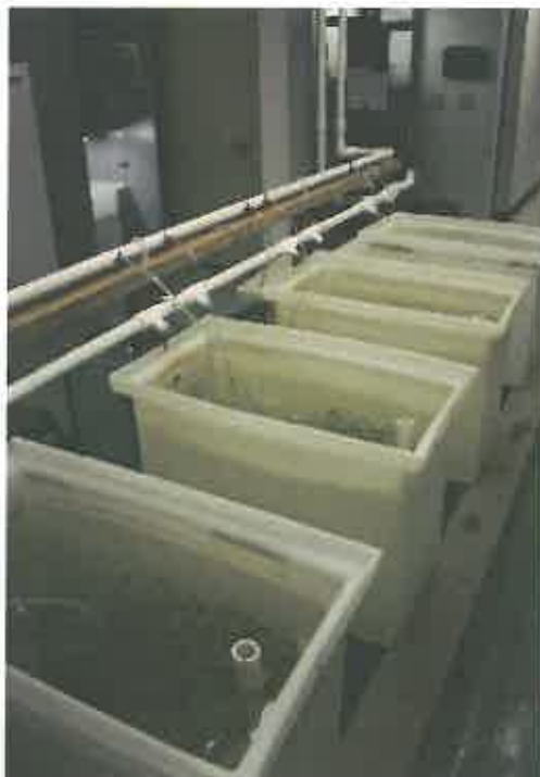
Fish are exposed to final effluent for toxicity testing.
