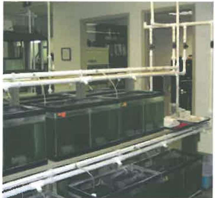
Fish are exposed to final effluent for toxicity testing.
