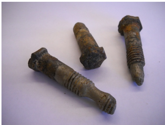
Corroded Valve Bolts
