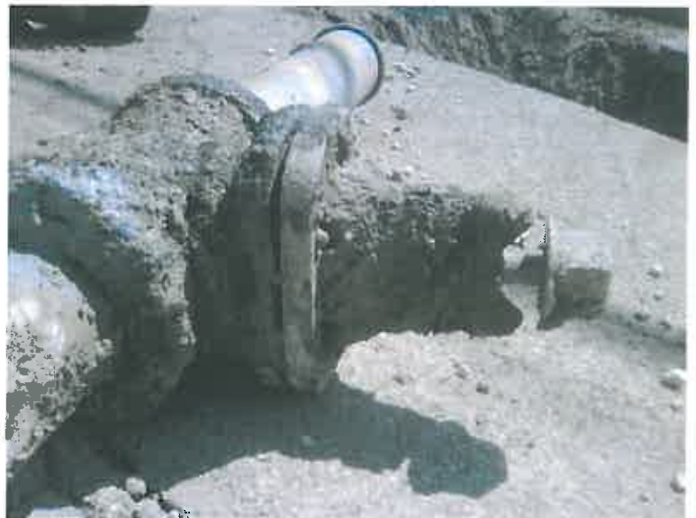
Separation of the Valve Bonnet from the Valve Body
